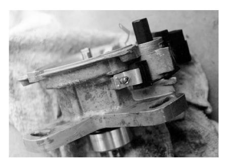
For your reference, this is the screw that necessitated the removal of my distributor. When the distributor is mounted in the car, this screw is tricky to get at and, of course, I buggered it up trying.
