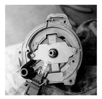
Assembly is basically the reverse of assembly. Make sure the distributor housing is clean. Smear a small amount of heatsink compound on the coil and place it in the housing as shown. Don't overdo the compound - too much is worse than not enough.
