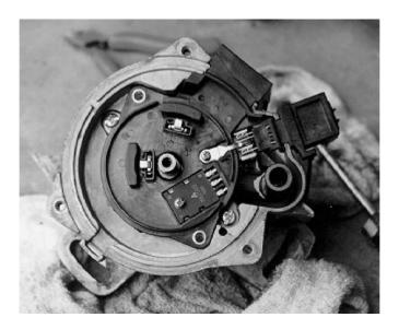
Smear a little heatsink grease onto the back of the igniter where it contacts the distributor housing. Try not to get any into the mounting holes.
