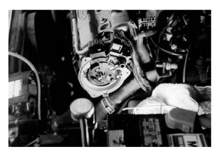
Remove the Philips screw in the center of the distributor shaft and remove the rotor support piece from the shaft. The interrupter assembly is a snug fit on the shaft so it might take some wiggling to get it off. Once the interrupter wheel assembly is off, pull out the wheel spacer behind it.
